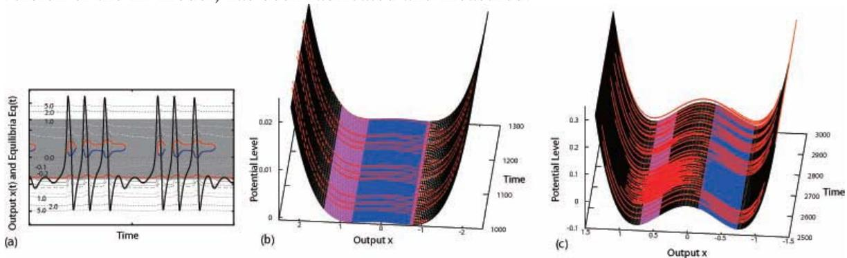
**Fig. 1** Burst and chaotic oscillations bound by the potential with the active areas. (a) Time series of output on a contour map of the potential. Bird's eye views of outputs on the potentials, (b) for a burst oscillation and (c) for a chaotic oscillation.
